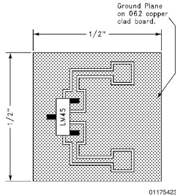
**FIGURE 3. Printed Circuit Board Used for Heat Sink to Generate All Curves.
