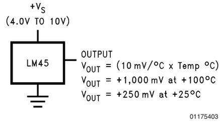
**FIGURE 1. Basic Centigrade Temperature Sensor (+2.5°C to +100°C)**
